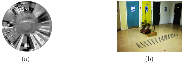
Figure 11: First initial position. (a) Difference between the desired and initial omnidirectional images. (b) Initial position of the robot with the desired one as a ghost (Figure 10(b)).
