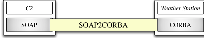
Fig. 6. Pairwise mediation between layered protocols
