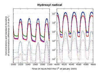
**Fig. 4.** Time evolution of the horizontal mean over the whole domain of OH hourly concentrations for different levels (ground level in green, third level in blue and top level in red). Full lines are used for a priori simulations and crossed ones are used for a posteriori simulations. The dotted lines represent the standard deviation computed for the corresponding levels.
