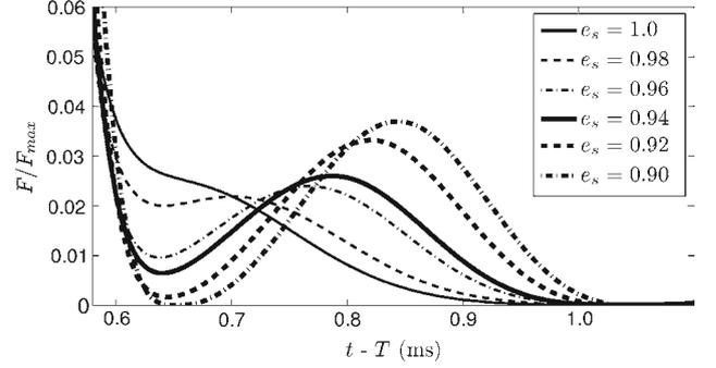
**Fig. 25** Secondary solitary waves (SSWs) obtained numerically for the even chain with different values of the restitution coefficient  $e_s$ . The force  $F$  is computed at the left contact of bead 17 and is normalized by the maximal value. The time origin corresponds to the maximal force
