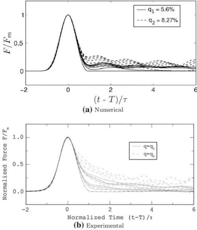
**Fig. 12** Collapse of the pulses presented in Figs. 10 and 11 when the force is normalized to the amplitude  $F_m$ , and the time scale is  $(t - T)/\tau$  where  $T$  and  $\tau$  are the measured time of flight and pulse duration, respectively. **a** for the numerical data and **b** for the experimental data extracted from figure 4 in [34]
