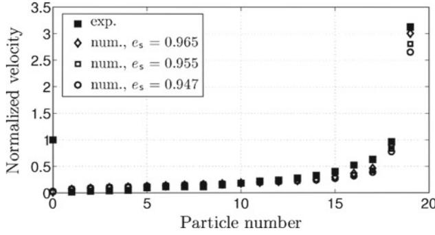
**Fig. 6** Post-impact velocity of the beads, normalized by the impact velocity, obtained in the experimental tests and in the numerical simulations with different values for the restitution coefficient  $e_s$ . The experimental data are extracted from figure 6.a in [36]
