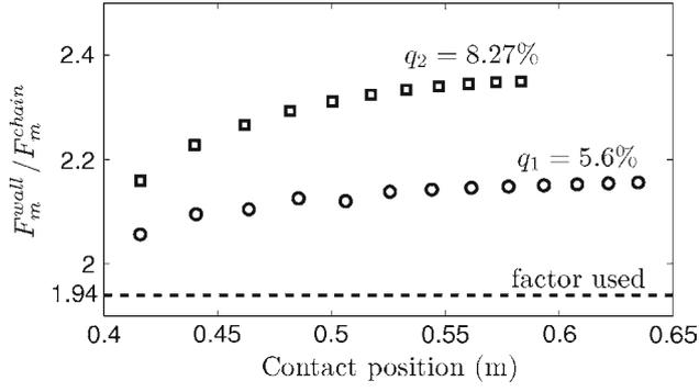
**Fig. 14** Scaling factor for the force amplitude versus contact position obtained from the numerical simulation for the two tapered chains with  $q_1 = 5.6\%$  and  $q_2 = 8.27\%$ , compared to the one used in (21)
