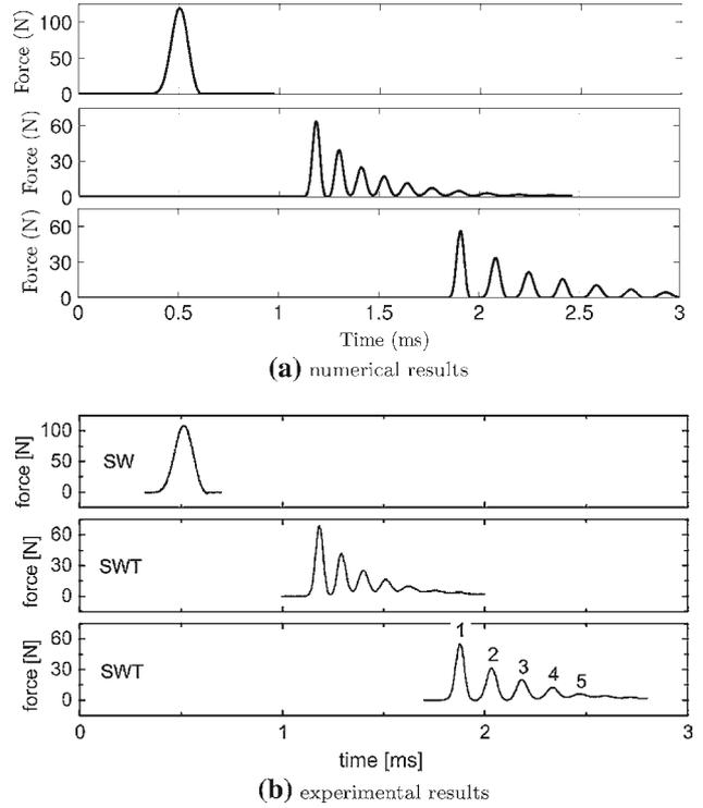
Fig. 20 Solitary wave and solitary wave trains in stepped chains obtained from **a** the numerical simulations and **b** from the experimental tests in [23]. The first row corresponds to the force pulse recorded at the end of the monodisperse chain composed of 7 large beads. The second and last rows correspond to the force pulses recorded at the end of the stepped chains with 25 and 50 small beads, respectively
