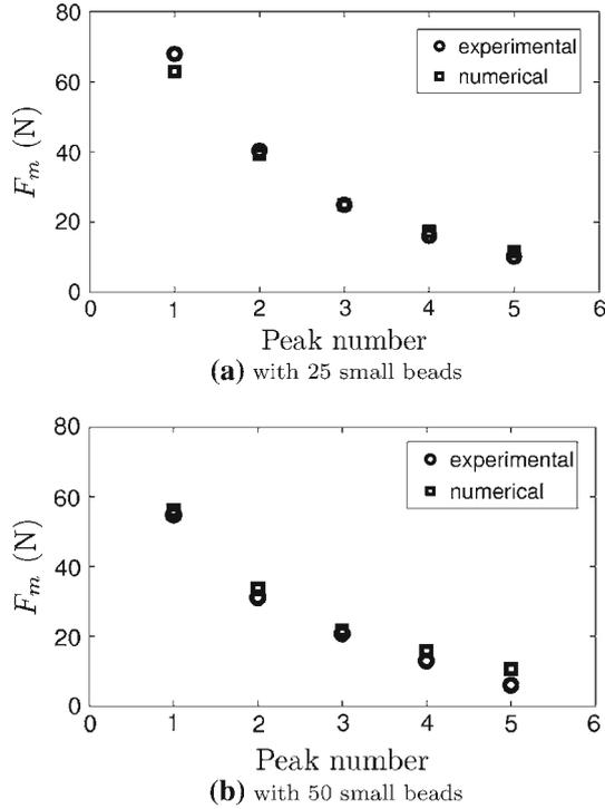
**Fig. 21** Amplitude of single solitary waves in the solitary wave trains obtained from the numerical simulations, compared to the experimental data extracted from figure 2 in [23] for the solitary wave trains at the end of the stepped chains with **a** 25 and **b** 50 small beads
