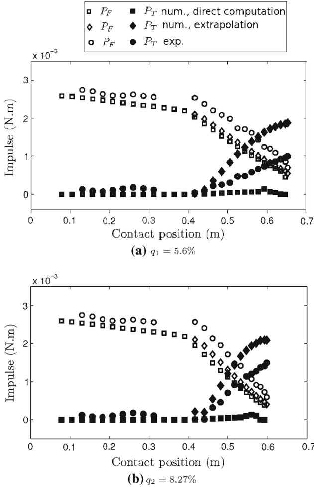
**Fig. 17** Front and tail impulses  $P_F$  and  $P_T$  versus the contact position obtained from the numerical simulations with the extrapolation and the direct computation method (represented by symbols *diamond* and *square*, respectively) compared to the experimental data (represented by symbol *circle*). **a** for  $q_1 = 5.6\%$  and **b** for  $q_2 = 8.27\%$ . The experimental data are extracted from figure 5 (d1 and d2) in [34]
