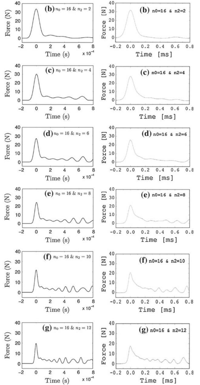
**Fig. 11** Force pulses at the rigid wall obtained from the numerical tests  $T_1$  for different tapered sub-chains with  $n_2 = 0, 2, 4, 6, 8, 10, 12$  (left column) and from the experimental tests (right column) for  $q_2 = 8.27\%$ . The experimental data are extracted from figure 2 in [34]
