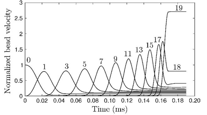
**Fig. 5** Velocity of different beads, normalized by the impact velocity, versus time during the impact process resulting from the numerical simulation of the tapered chain considered in [36] with  $e_s = 0.965$ . The number above each curve corresponds to the bead number
