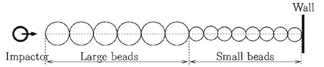
Fig. 19 Impact tests on stepped chains in [23]
