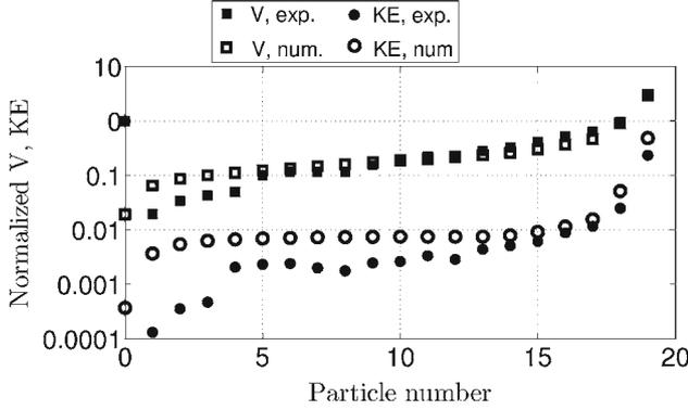
**Fig. 7** Post-impact velocity ( $V$ ) and kinetic energy (KE) of the beads (normalized by the respective initial values of the impactor) plotted in the semilog scale, obtained in the experimental tests and in the numerical simulations with the restitution coefficient  $e_s = 0.965$ . The experimental data are extracted from figure 6.b in [36]
