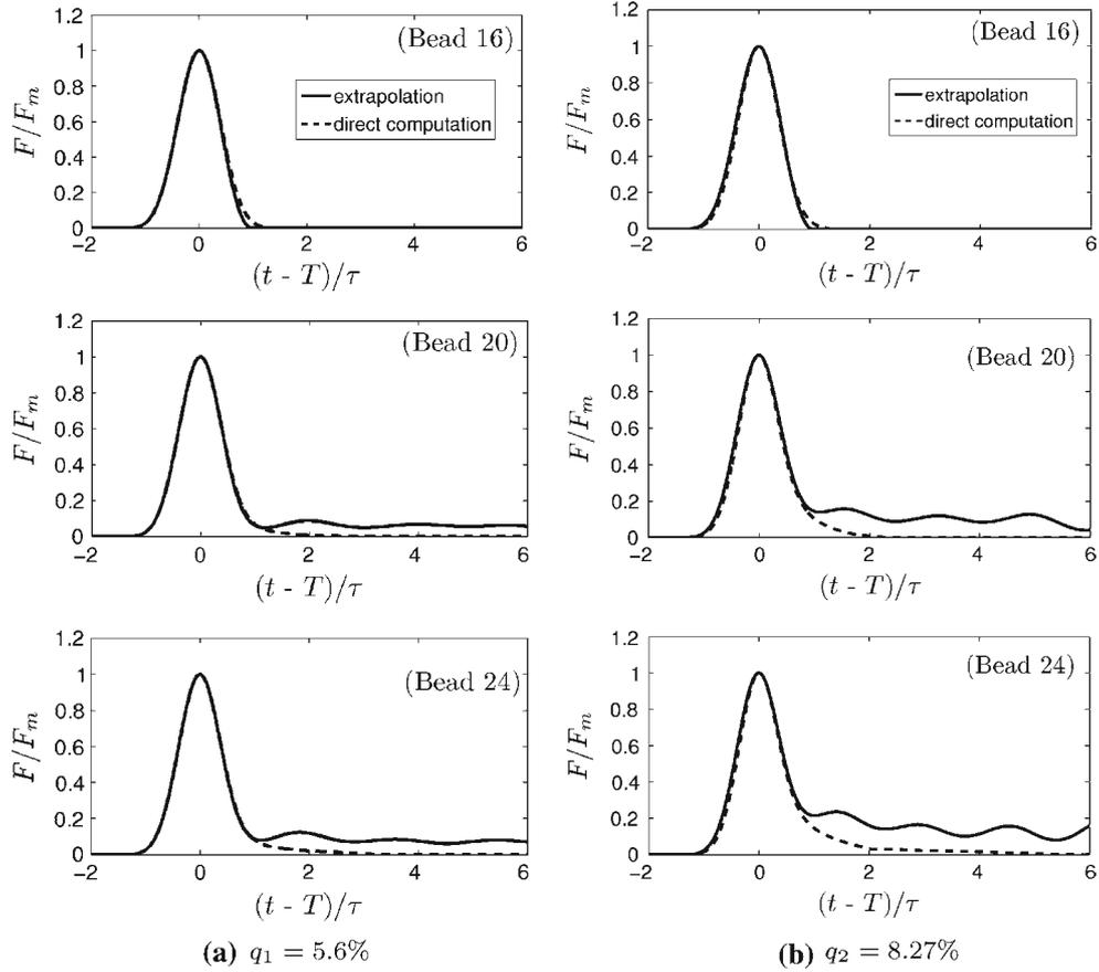
**Fig. 18** Overlap of normalized force pulses at the right contact of beads 16, 20, 24 in the considered tapered chains obtained by the extrapolation and direct computation methods. Force pulses are normalized by their amplitude and the time scale is  $(t - T)/\tau$ . **a** for  $q_1 = 5.6\%$  and **b** for  $q_2 = 8.27\%$
