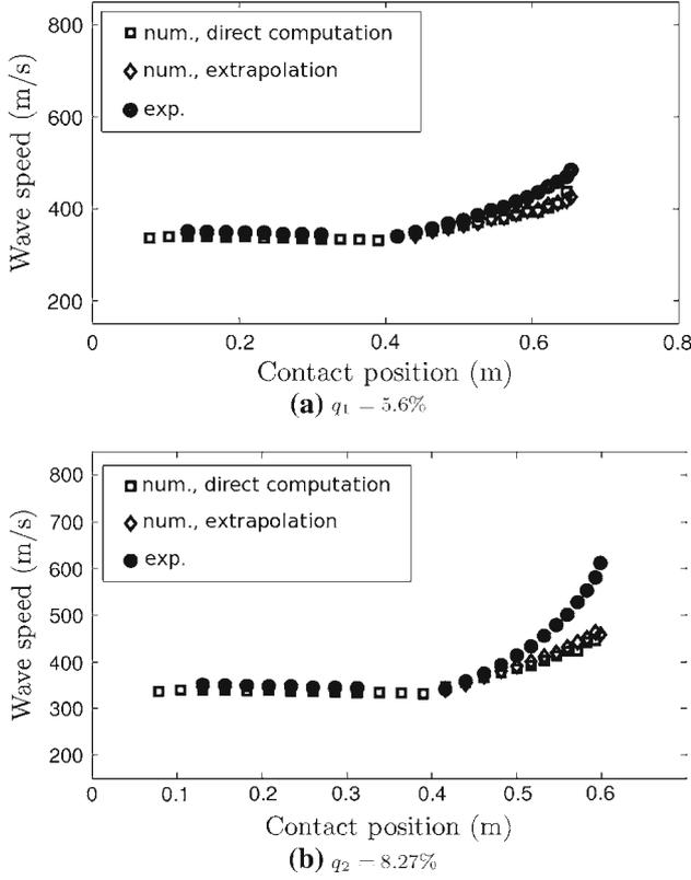
**Fig. 16** Wave speed versus the contact position obtained from the numerical simulations with the extrapolation and direct computation methods (represented by symbols *diamond* and *open square*, respectively), compared to the experimental results (represented by symbol *filled circle*). **a** for  $q_1 = 5.6\%$  and **b** for  $q_2 = 8.27\%$ . The experimental data are extracted from figure 6 (c1 and c2) in [34]
