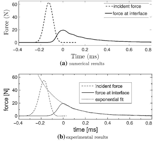
**Fig. 22** The incident force and the interfacial force obtained from **a** the numerical simulations and **b** from the experimental tests performed in [23]. The experimental data are extracted from figure 3.a in [23]
