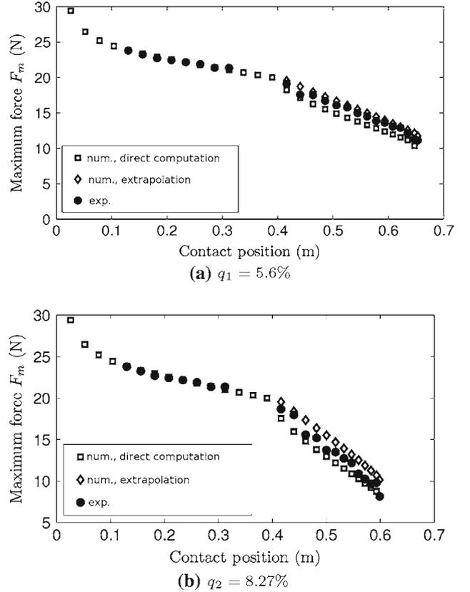
**Fig. 13** Force pulse amplitude versus the contact position obtained from the numerical simulations by both extrapolation and direct computation methods (represented by symbols *diamond* and *open square*, respectively), compared to the experimental results (represented by symbol *filled circle*). **a** for  $q_1 = 5.6\%$  and **b** for  $q_2 = 8.27\%$ . The experimental data are extracted from figure 5 (b1 and b2) in [34]
