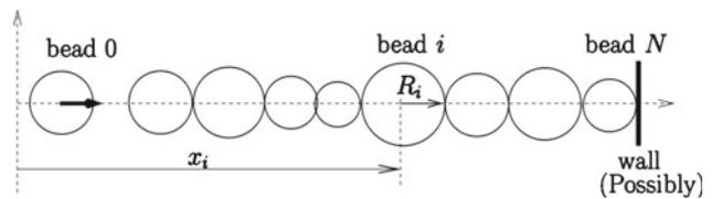
**Fig. 1** Configuration of a granular chain with possibly a rigid wall at the end, impacted by a striker (bead 0)
