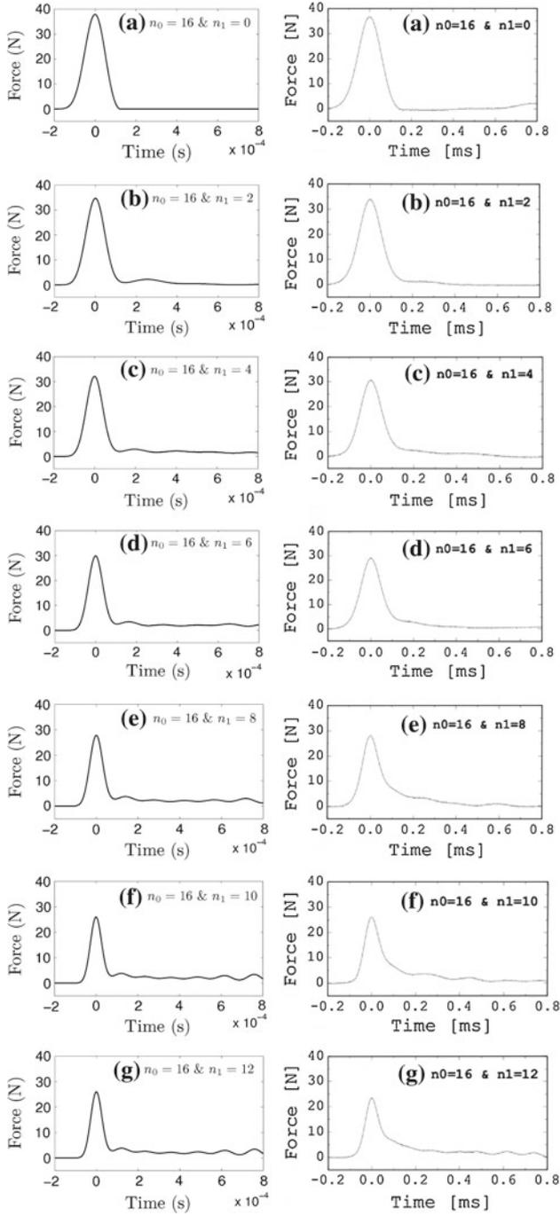
**Fig. 10** Force pulses at the rigid wall obtained from the numerical tests  $T_1$  for different tapered sub-chains with  $n_1 = 0, 2, 4, 6, 8, 10, 12$  (left column) and from the experimental tests (right column) for  $q_1 = 5.6\%$ . The experimental data are extracted from figure 1 in [34]
