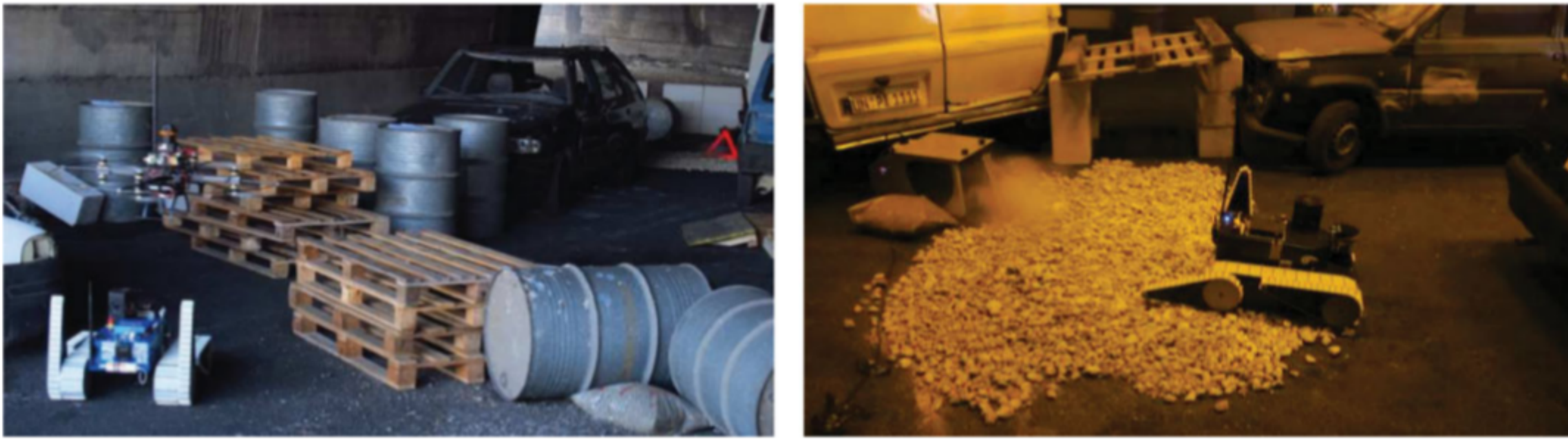
Fig. 1. (Colour online) Tunnel car accident at Montelibretti's firefighter Italian school used for USAR evaluation.
