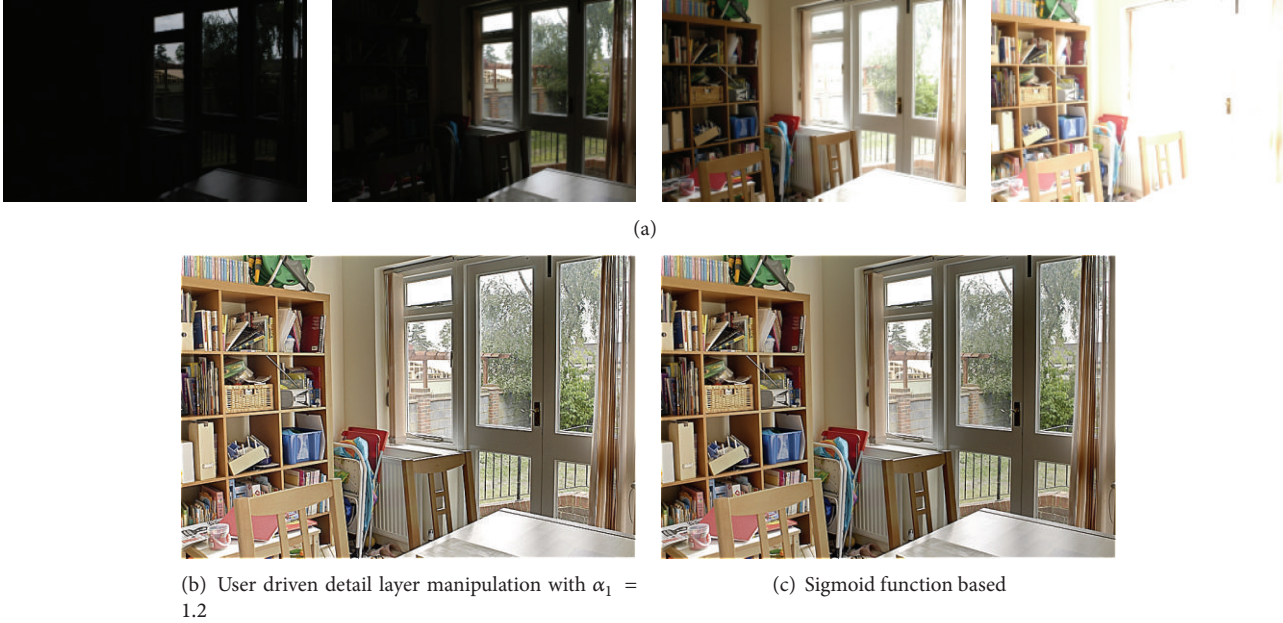
FIGURE 1: (a) Images representing multiple exposures; ((b), (c)) illustration of our detail-preserving exposure fusion result. Note that our result contains more details in brightly and poorly illuminated areas with natural contrast. The fine textures on the chair are accurately preserved. (c) Our detail layer enhancement based on sigmoid function across all the inputs reveals more texture details in the fused image and does not depict noticeable artifacts near strong edges.
