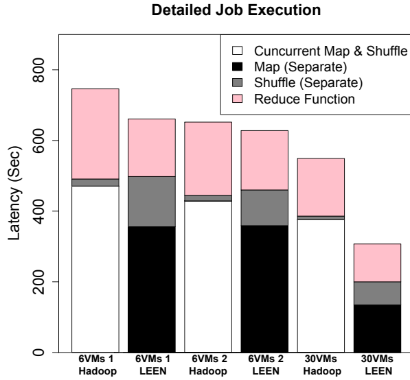
Fig. 8 Detailed performance of each stage in LEEN against native Hadoop for the three test sets
