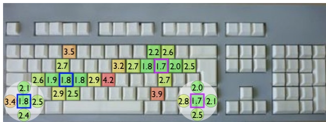
Figure 6. Heat map of selection speed (in s) for each target keys. The two raised keys are outlined. Insets show speeds for Top Push and the directional pushes on the raised keys.
