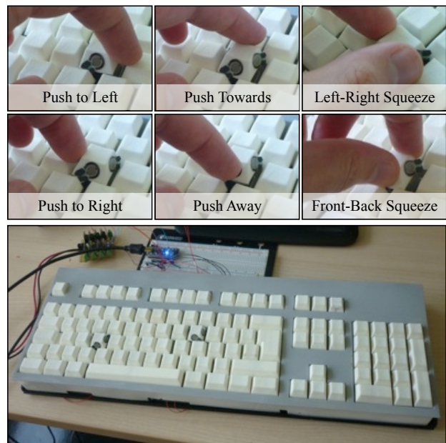
Figure 2. Top: the physical manipulations that can be detected on each key. Bottom: our Métamorphe prototype.
