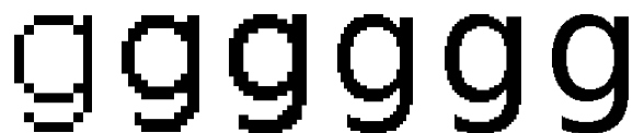
Figure 8. The same glyph rendered at different resolutions (16pt, 24pt, 32pt, 48pt, 64pt, and 128pt) without antialiasing.
