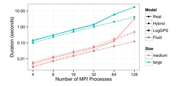
Figure 4: Comparison between simulated and actual execution times for the MPI\_Alltoall operation.
