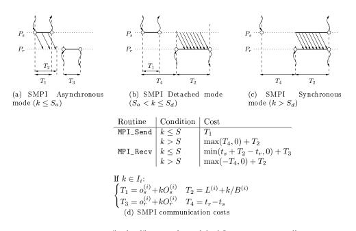
Figure 3: The "hybrid" network model of SMPI in a nutshell.
