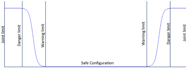
Fig. 1. Joint limit avoidance scheme
