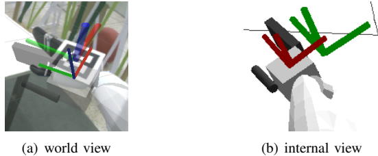
Fig. 12. The net effect of robot calibration errors on REEM's hand and the marker frame
