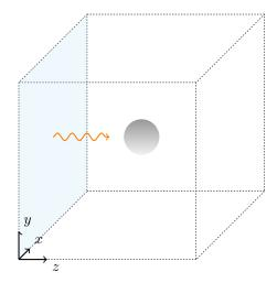
Figure 7 | Physical situation: gold nanosphere illuminated with a plane wave.
