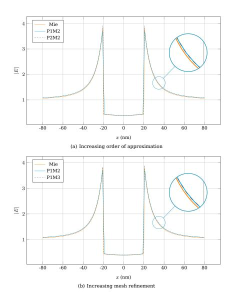
Figure 9 | Mie and DG 1D plot of the electric field modulus across the dispersive gold nanosphere for various meshes and approximation ordrers.
