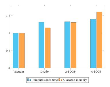
Figure 13  $\mid$  Computational time and memory allocation for the generalized dispersive formulation for various models.
