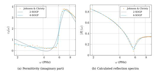
Figure 14  $\mid$  Comparison of the fitting of imaginary part of the permittivity silver by 2-SOGP and 4-SOGP and its impact on the prediction of the reflectance spectrum.
