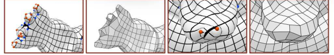
Figure 7: The ARMADILLO parametrized using MIQ without stiffening in 7.4s. Contains 78 flipped faces and two with zero area.
