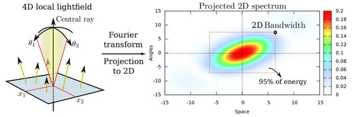
Fig. 2. *Left*: 4D local light field parametrization adopted by Durand *et al.* [2]. *Right*: 2D parametrization introduced by Soler *et al.* [15]. We define local bandwidth  $\nu \equiv [\nu_s \ \nu_a]^T$  (black dot) so that 95% of the spectral energy lies in the dotted rectangle.
