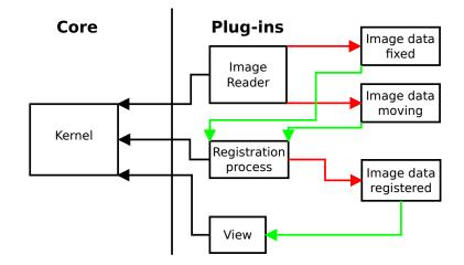
Figure 1: General architecture, here demonstrating an image reader, a view, and a registration plugin working together. (inputs are green, output red)
