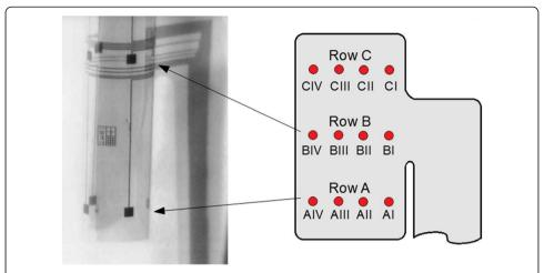
**Figure 3 A 12-contact cuff electrode.** A 12-contact cuff electrode the same as the one used in the experiments (left), and the symbols of the stimulating contacts used in the paper (right). Arrows indicate the location of rows A and B in the photograph. Row C is not visible.
