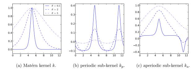
Figure 3: Examples of decompositions of a Matérn 3/2 kernel as a sum of a periodic and aperiodic sub-kernels. The three graphs on each plot correspond to a different value of the lengthscale parameter  $\theta$ . For this example the input space is  $D = [0, 4\pi]$ , the cut-off frequency is q = 20 and one of the variables of the kernels is arbitrarily fixed to 5.
