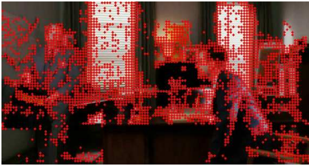
Fig. 3 Visualization of densely sampled feature points after removing points in homogeneous areas using the criterion in Eq. (1). We only show feature points in the first spatial scale. The sampling step size W is 5 pixels, which is the default setting in our experiments.
