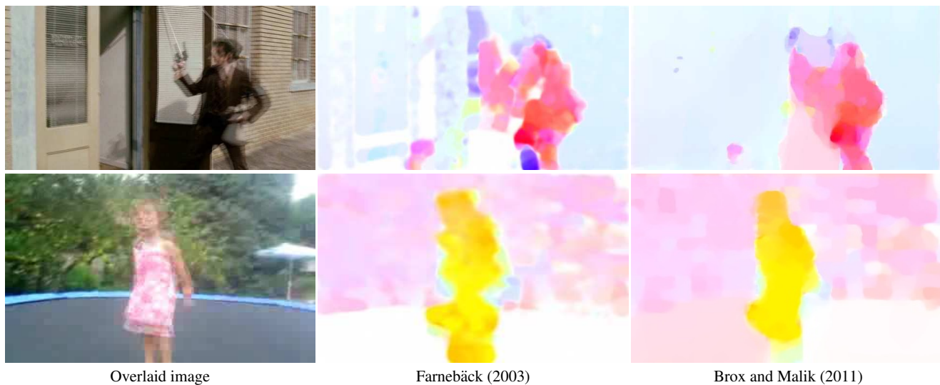
Fig. 10 Examples from Hollywood2 (top) and YouTube (bottom). The left column shows the overlaid image of two consecutive frames. The middle and right columns are the visualization of two optical flow methods Farneback (2003) and Brox and Malik (2011).
