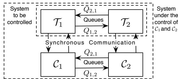
Figure 1: Control architecture of a distributed system.
