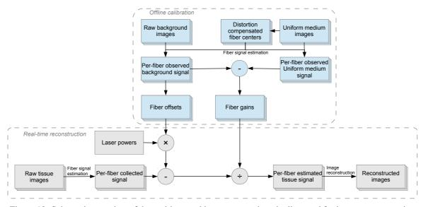
Figure 10: Schematic overview of the multispectral image computing pipeline used for image reconstruction
