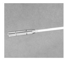
(b) Tip of the UltraM flexible optical miniprobe. It offers a lateral resolution of 1.4  $\mu m$ , a field of view of 240  $\mu m$  with an outer diameter of 2.6 mm
