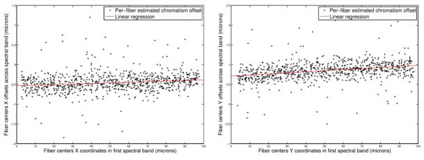
(a) Residual chromatic distortions on the horizontal (*x*) coordinate and linear regression fit
