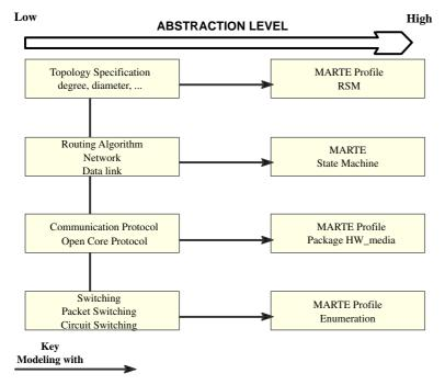
Fig. 5 Design flow for NoC modeling
