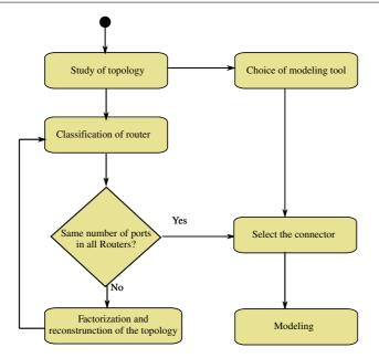
Fig. 6 Methodology for modeling NoC topologies
