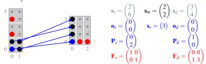
Note that, in principle, such a reshape relation can relate only a part of the elements of the source array with part of the elements of the destination array and that the source array can be the same as the destination array. We will use this possibility a lot in the following.
