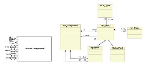
Fig. 11 Entity of the hardware router and related metamodel concept.
