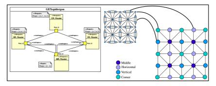
Fig. 9 Compact modeling of the GEXspidergon topology: one component by router degree and reshape connectors
