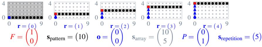
This figure represents the tiles for all the repetitions in the repetition space, indexed by  $r$ . The paving vectors drawn from the origin  $o$  indicate how the coordinates of the reference element  $\mathbf{ref}_{\mathbf{r}}$  of the current tile are computed. Here the array is tiled row by row.
