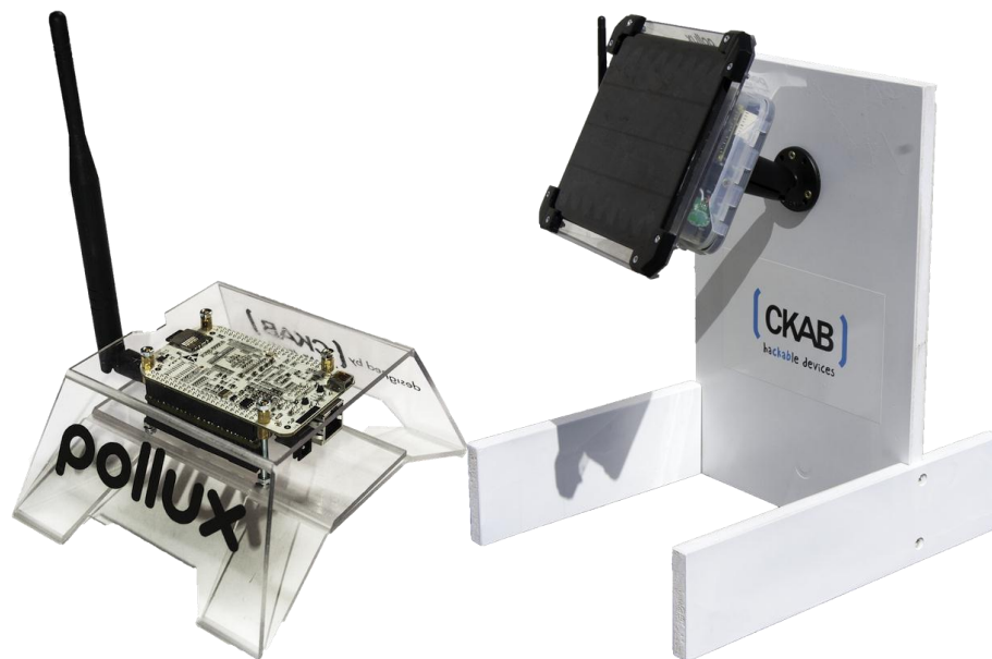
Figure 54: Pollux green station (gateway module and sensors)
