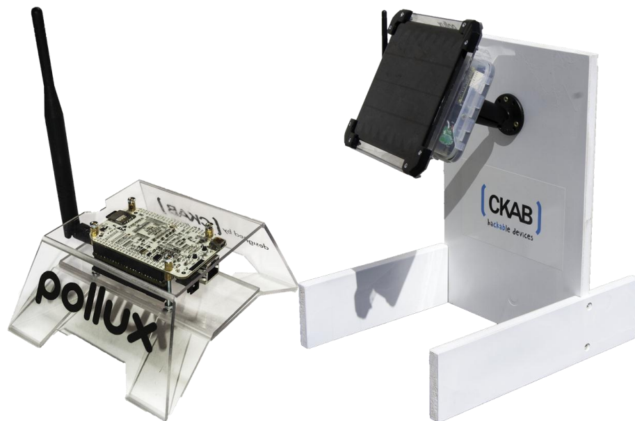
Figure 54: Pollux green station (gateway module and sensors)
