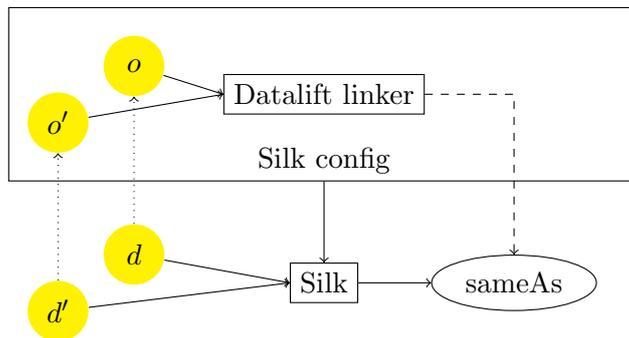
Figure 3.2: Integrating a linker directly within Silk.
