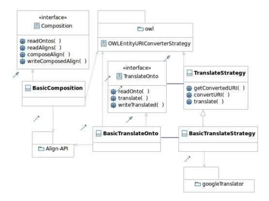
Figure 1: Class diagram for Multi-Align API.
