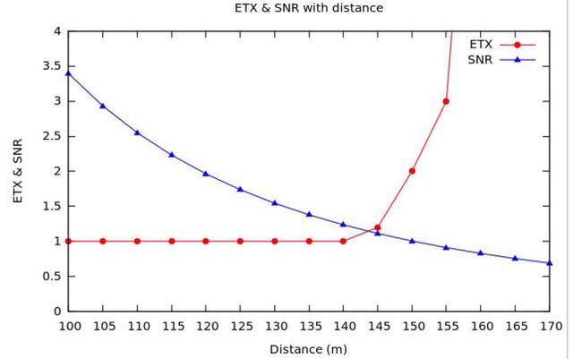
Fig. 2. SNR as function of the distance.
