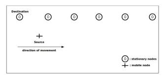
Fig. 4. Scenario 1: a mobile node passes along a fixed chain of nodes at a constant speed. There are 12 nodes: 11 stationary nodes, each placed at a distance of 100 meters forming a chain, and a mobile node.
