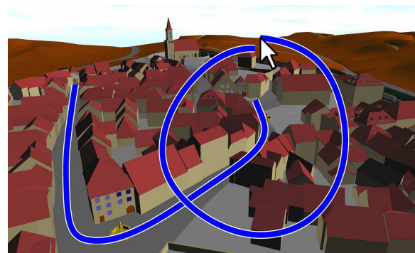
Figure 5: Example of a sketch-based navigation from [HD08]: the user draws a curve on the street and combines this command with a circle like gesture; the derived animation will move the camera along the sketched path and rotate for inspecting the target area.
