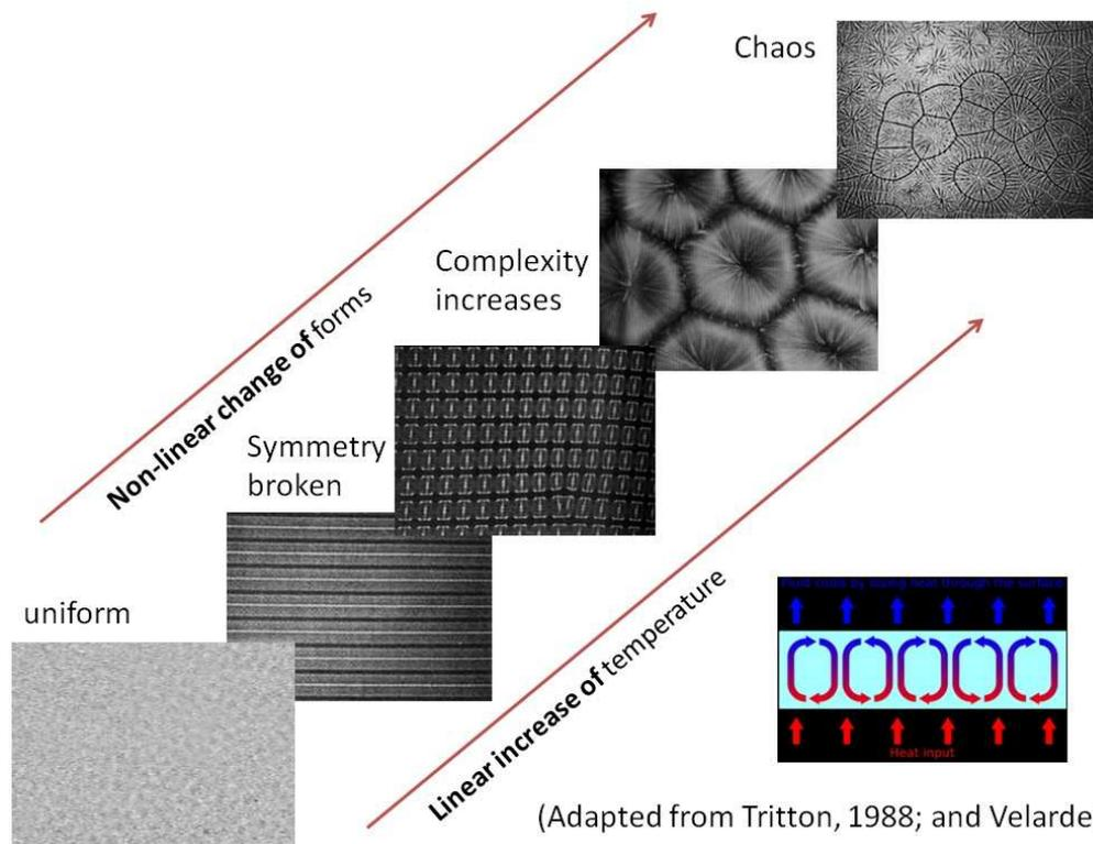
**Figure 2 Rayleigh-Bénard cells: when one heats from below a thin layer of oil spread out on a plane surface, convection currents with peculiar geometric shapes (lines or polygons) self-organize and these shapes change brutally when the temperature goes over given thresholds. This kind of non-linearity characterized many self-organized systems both in the inorganic and in the living world<sup>1</sup>.**
