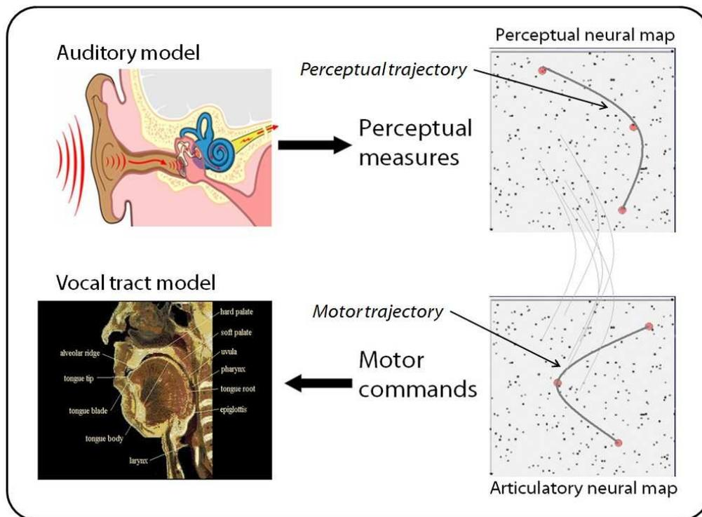
**Figure 4: The robot architecture in the artificial system. Each robot is equipped with an artificial ear, an artificial vocal tract, and two neural maps (perceptual and motor) that couple the ear and the vocal tract.**
