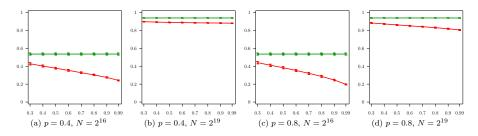
Figure 8: Waste (y-axis) as a function of the recall (x-axis) for a fixed precision (p = 0.4 and p = 0.8) and for a Weibull distribution (k=0.5).
