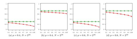
Figure 7: Waste (y-axis) as a function of the recall (x-axis) for a fixed precision (p = 0.4 and p = 0.8) and for a Weibull distribution (k=0.7).
