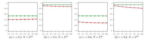
Figure 6: Waste (y-axis) as a function of the precision (x-axis) for a fixed recall (r = 0.4 and r = 0.8) and for a Weibull distribution of faults (with shape parameter k = 0.5).
