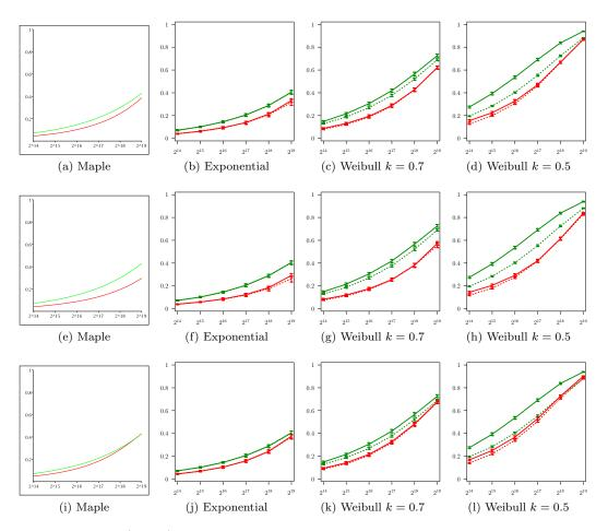
Figure 10: Waste (y-axis) for the different heuristics as a function of the platform size (x-axis), with p = 0.4, r = 0.7,  $C_p = C$  (first row),  $C_p = 0.1C$  (second row), or  $C_p = 2C$  (third row) and with a trace of false predictions parametrized by a uniform distribution.
