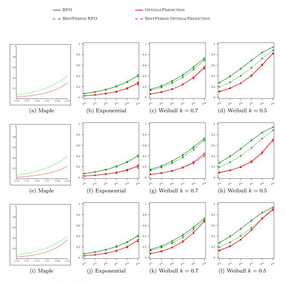
Figure 3: Waste (y-axis) for the different heuristics as a function of the platform size (x-axis), with p = 0.82, r = 0.85,  $C_p = C$  (first row),  $C_p = 0.1C$  (second row), or  $C_p = 2C$  (third row) and with a trace of false predictions parametrized by a distribution identical to the distribution of the trace of failures.
