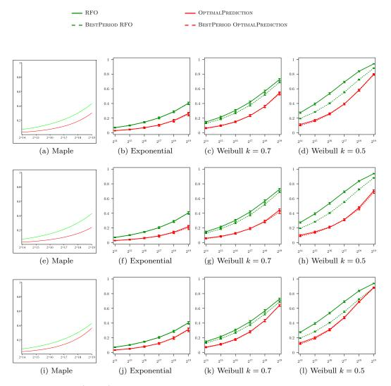
Figure 9: Waste (y-axis) for the different heuristics as a function of the platform size (x-axis), with p = 0.82, r = 0.85,  $C_p = C$  (first row),  $C_p = 0.1C$  (second row), or  $C_p = 2C$  (third row) and with a trace of false predictions parametrized by a uniform distribution.
