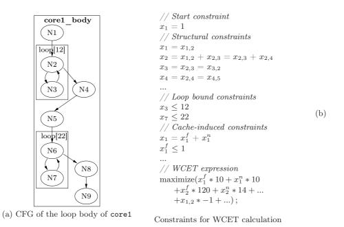
FIGURE 3 – State-of-the-art WCET calculation on the loop body of core1 in our illustrating example.
