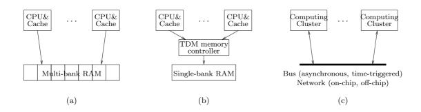
FIGURE 2 – Examples of execution platforms allowing simple contention avoidance : (a) Shared multi-bank RAM (, (b) Shared single-bank RAM with TDMA arbiter, (c) Distributed, NUMA, or network-on-chip architecture (computing cluster = a or b).
