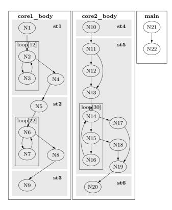
FIGURE 4 – Original control flow graph for the toy example. Shaded areas represent task portions between communications (subtasks)
