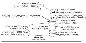
Figure 5. Automaton for the provisioning policy.
