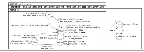
Figure 7. BZR program for coordination policy between provisioning and admission controller.
