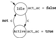
Figure 6. Automaton for the admission controller.
