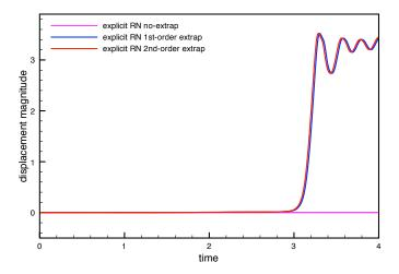
Figure 13: Comparison of the implicit and Robin-Neuman explicit coupling schemes: interface mid-point displacement magnitude of the bottom structure vs. time.
