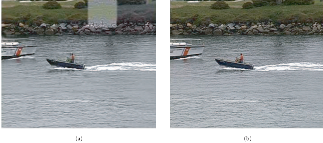
FIGURE 21: A sample of video stream at the receiver, (a) transmitted by media-oriented algorithm with 0.1% bit errors (SNR = 1.3, rate = 12 Mbps), (b) original video stream.
