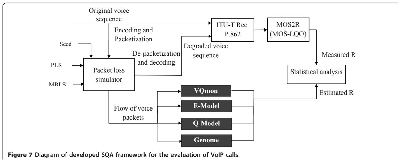
**Figure 7** Diagram of developed SQA framework for the evaluation of VoIP calls.
