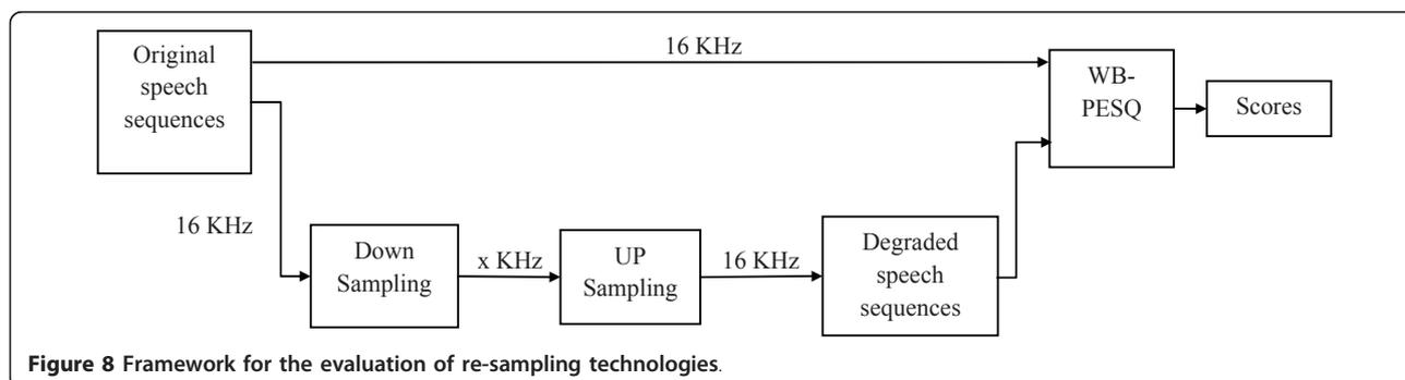
Figure 8 Framework for the evaluation of re-sampling technologies.
