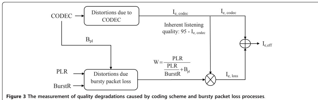
**Figure 3** The measurement of quality degradations caused by coding scheme and bursty packet loss processes.
