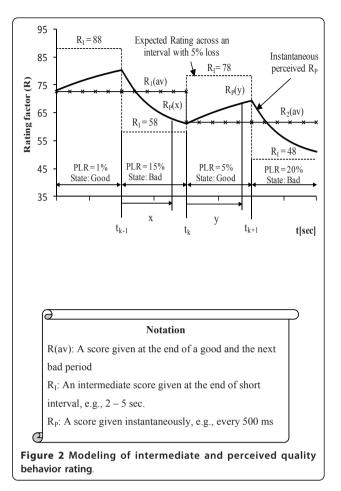
evolution of  $R_{\rm I}$  (dashed line) and  $R_{\rm P}$  (solid line) as function of time and channel state during a presented speech sequence.
