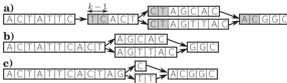
**Figure 2 Graph simplification.** Graph simplification (Algorithm 1, Step 15). **a)** the graph before simplification. **b)** After removing the first  $k - 1$  characters of each internal node and after merging non branching nodes. **c)** After common prefix and suffix factorizations.
