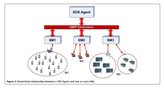
In fact, the SM abstracts the hardware features of sensing devices, the communication technologies, and the topologies for communications among sensors. The communication between SMs and the SOS Agent is based on the XMPP communication protocol. XMPP is widely used (see GTalk chatting protocol of Google) and very flexible (contrary to other messaging/signalling protocols, e.g., SIP) since it offers:
