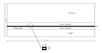
FIGURE 2. Nuclear waste repository and surrounding geological layers.
