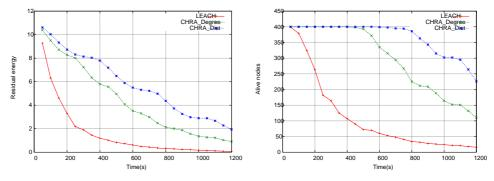
(a) Residual energy in of time (400 node net- (b) Number of alive nodes in time (400 node work and density 0.11) network and density 0.11)
