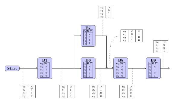
Figure 14: Illustration of the relative cache states.
