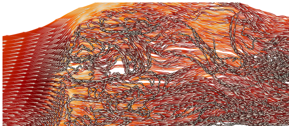
Figure 7: Streamlines depicted through light gray arrow shapes combined with a halos colored with a color map to depict velocity.
