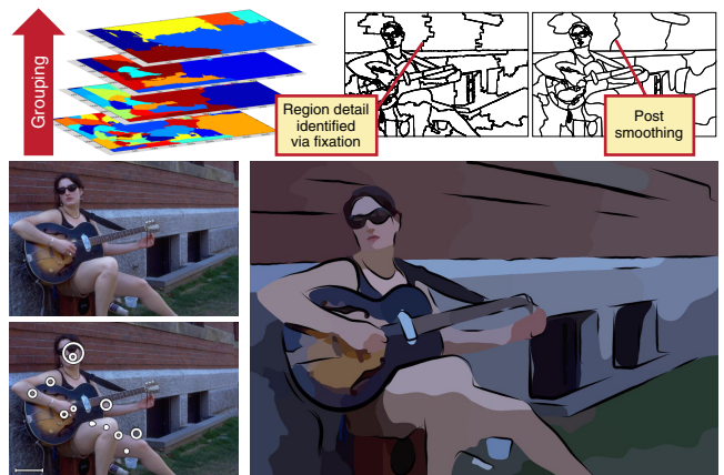
Fig. 5. Interactive abstraction system of DeCarlo and Santella [29]. Images are segmented in a scale-space pyramid (top-left). The viewer’s gaze is drawn to particular image regions; these regions are locally decomposed into finer segments traversing the pyramid (bottom). Outlines are smoothed and superimposed to delineate region boundaries (top-right).
