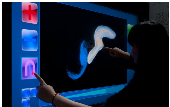
Fig. 1: Lasso-based selection interaction on the 2D touch surface to obtain a selection in 3D space [11].
