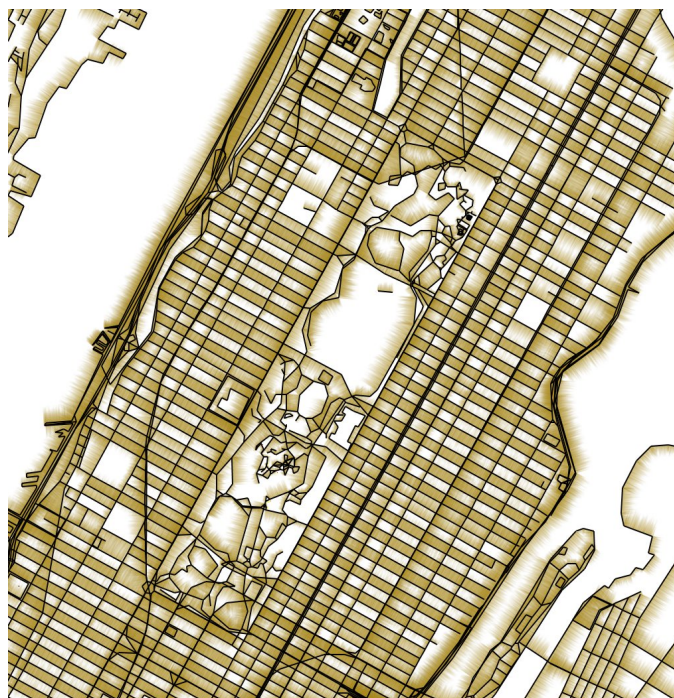
Figure 14. Manhattan with Central Park, simplified with Ramer-Douglas-Peucker to about \frac{1}{2} of the original edge count.
