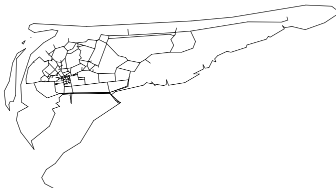
Figure 7. Map from Figure 3 after simplification with the Ramer-Douglas-Peucker technique to 452 edges.
