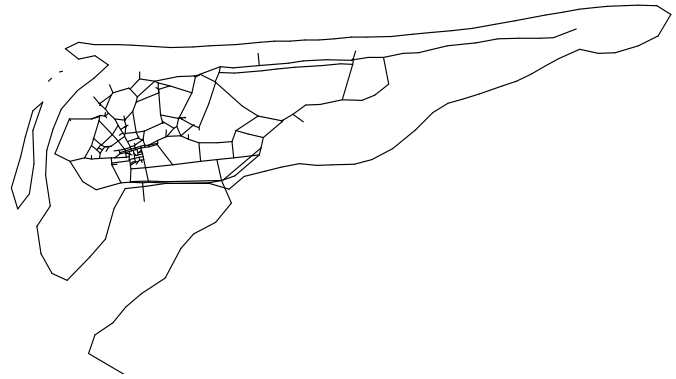
Figure 4. Map from Figure 3 after simplification from 2086 edges to 452 edges using progressive meshes, with intersections and end nodes pinned to their original locations.
