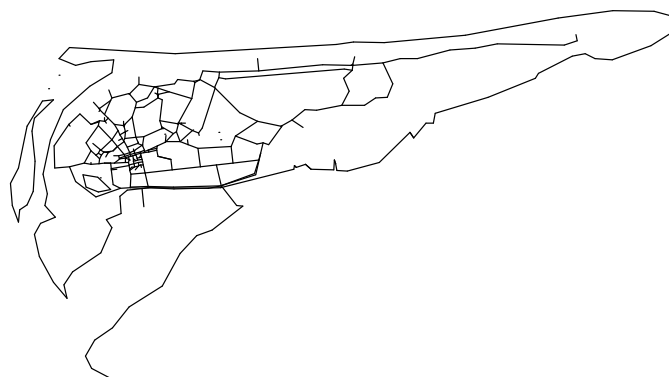
Figure 8. Map from Figure 3 after simplification with the Visvalingam-Whyatt technique to 452 edges.
