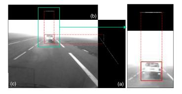
Fig. 9. Result of (a) "v-disparity" image (b) "u-disparity" image computations using our modified quasi-dense matching algorithm. (c) This leads to the computation of robust and precise bounding boxes around obstacles without any arbitrary thresholds.
