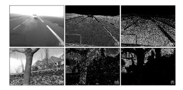
Fig. 6. Comparison of roughness of (a) our road image under foggy weather; (b) image used by Lhuillier; (c)(d) white pixels x where 0 < s(x) < 0.05; (e)(f) white pixels x where 0 < s(x) < 0.01.
